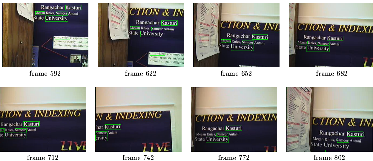
Fig. 11. Tracking algorithm applied to scene text with erratic motion in “poster.mpg” video sequence.
