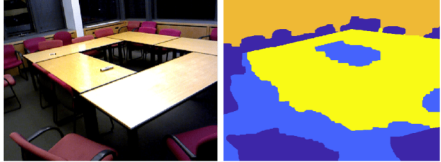
Fig. 1: We automatically annotate indoor scenes for training semantic segmentation models. Images (left) are automatically annotated (right) based on off-the-shelf object detectors and a 3D room layout estimator.
