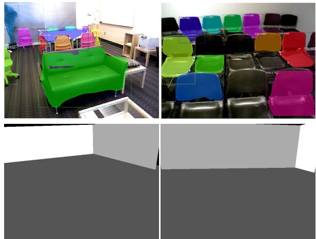
Fig. 4: Sample detection and 3D room layout results from two different scenes: Studyroom (Left) and MIT-32 (Right) from SUN3D [17]. Detector outputs (top) from Mask RCNN [10] provide an initial coarse segmentation around detected objects, while 3D layout estimation (below) explains background categories including “wall,” “floor,” and “ceiling.”
