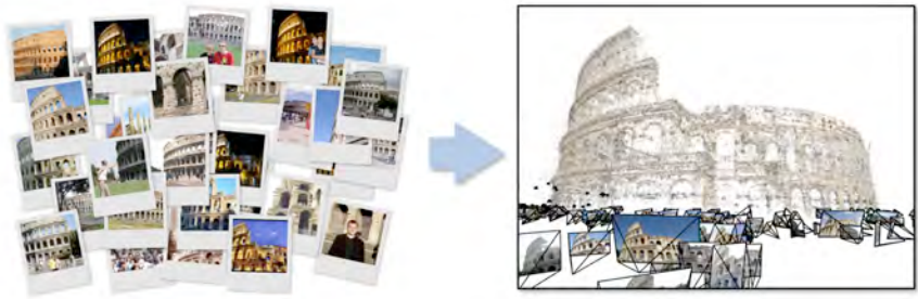
Fig. 2. From an unstructured collection of photographs downloaded from Flickr (left), we can produce a 3-d model of the original scene (right). (© Noah Snavely)
