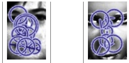
Figure 2.3: Detected SURF features for a human face (left) and avatar face (right).
