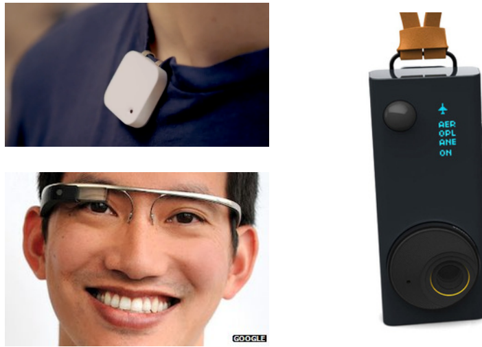
Figure 5.1: Wearable camera devices. Clockwise from top left: Narrative Clip takes photos every 30 seconds; Autographer has a wide-angle camera and various sensors; Google Glass features a camera, heads-up display, and wireless connectivity. (Photos by Narrative, Gizmodo, and Google.)
