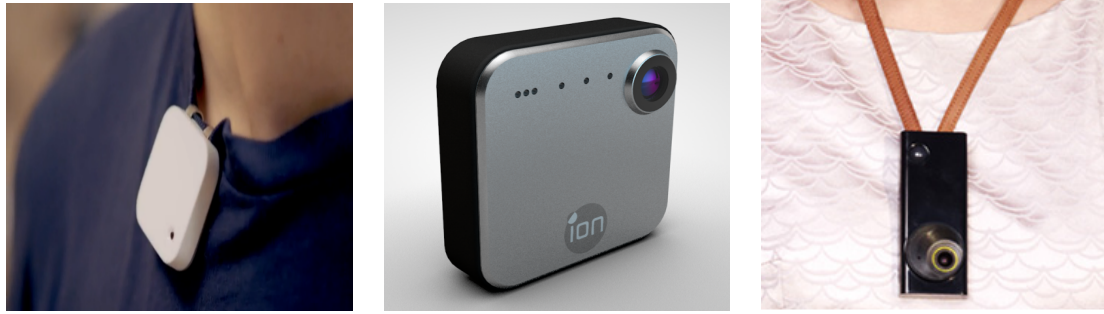
Figure 1.6: Wearable camera devices. Left: Narrative Clip takes photos every 30 seconds; Middle: iON snap camera captures images as well as videos. Right: Autographer has a wide-angle camera and various sensors; (Photos by Narrative, Gizmodo, and Gizmag.)
