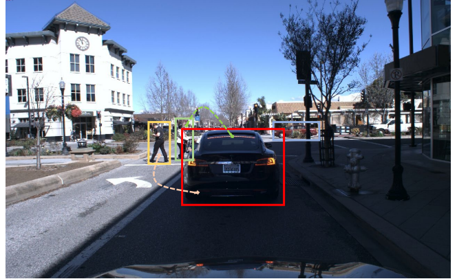
Fig. 1: Given a video clip, our goal is to estimate, in an online fashion, which objects in the last frame are important for the driver to make real-time control decisions. We also visualize different candidate object boxes, while the red box is the ground truth. Without considering the interaction between pedestrians and the front car, traditional methods make mistakes by predicting both pedestrians and the front car as important. Our proposed method can effectively model the interactions among other objects (visualized as dashed arrows) with a novel interaction graph and thus make the correct prediction. In this example, the front car prevents the ego vehicle from hitting the pedestrians and thus reduces the importance of them.
