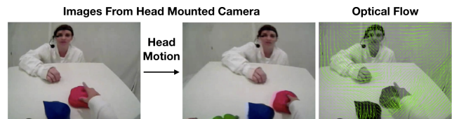
Figure 1: We estimate angular head motion in egocentric video, using both visual content and optical flow.
