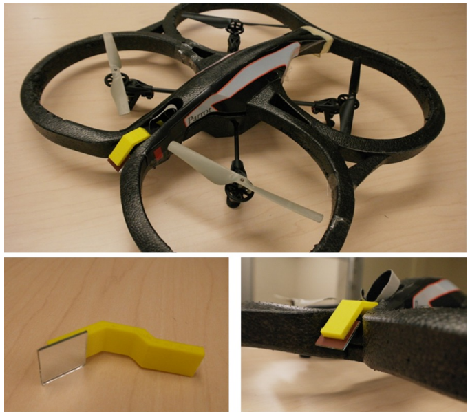
Fig. 2. We use the Parrot AR.Drone2.0 as our hardware platform (top), adding a mirror to the front-facing camera in order to detect objects on the ground (bottom).
