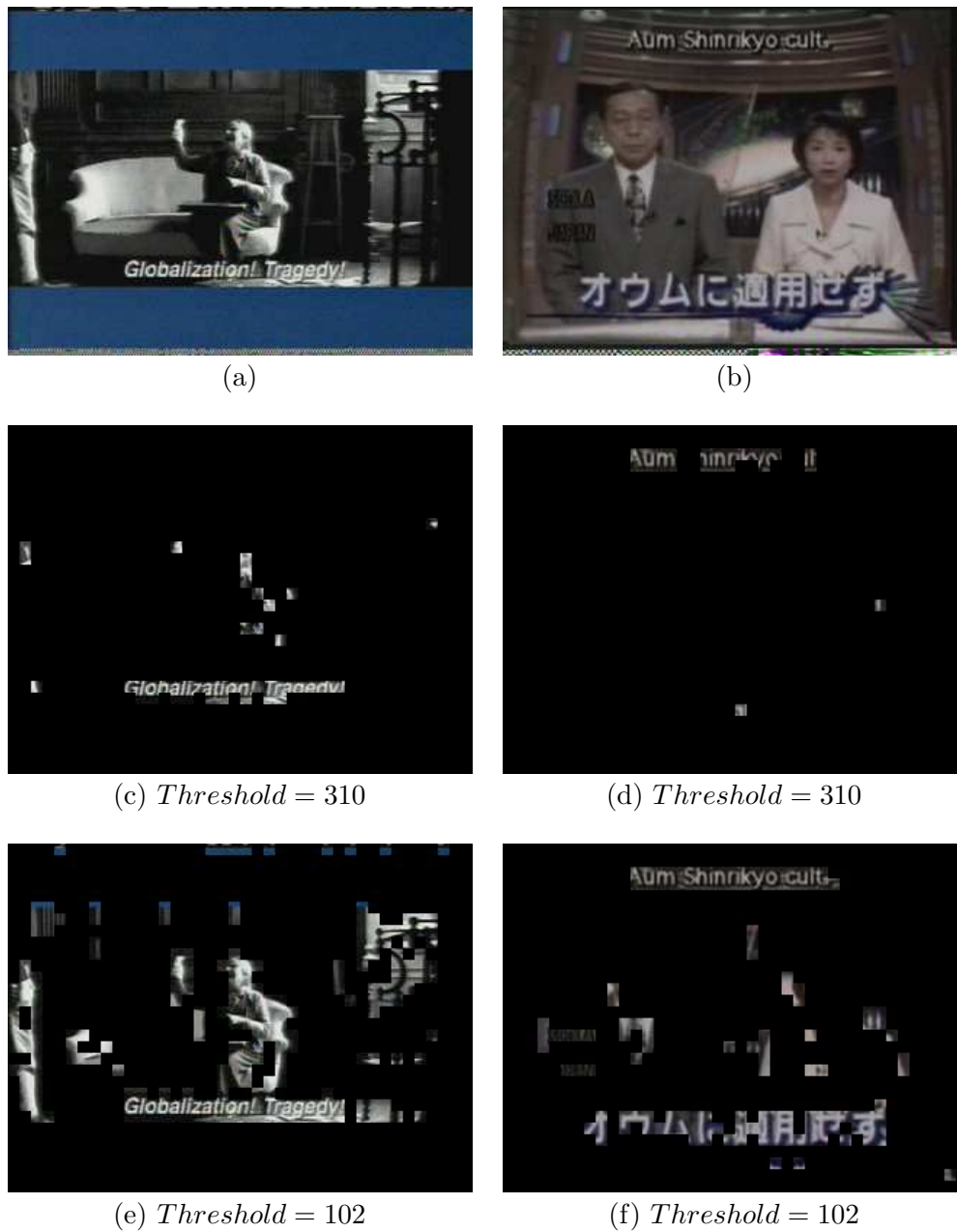
Fig. 2.1. Text block detection by thresholding DCT coefficient energies. (a) and (b): Two sample video frames. (c) and (d): Results of detection with threshold at 310. (e) and (f): Results of detection with threshold at 102.
