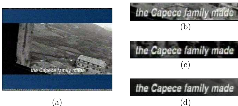
Fig. 4.4. Temporal averaging reduces background noise and improves contrast. (a): sample frame from a video sequence; (b) and (c): localized text region in two frames of the sequence; (d): result of temporal averaging.
