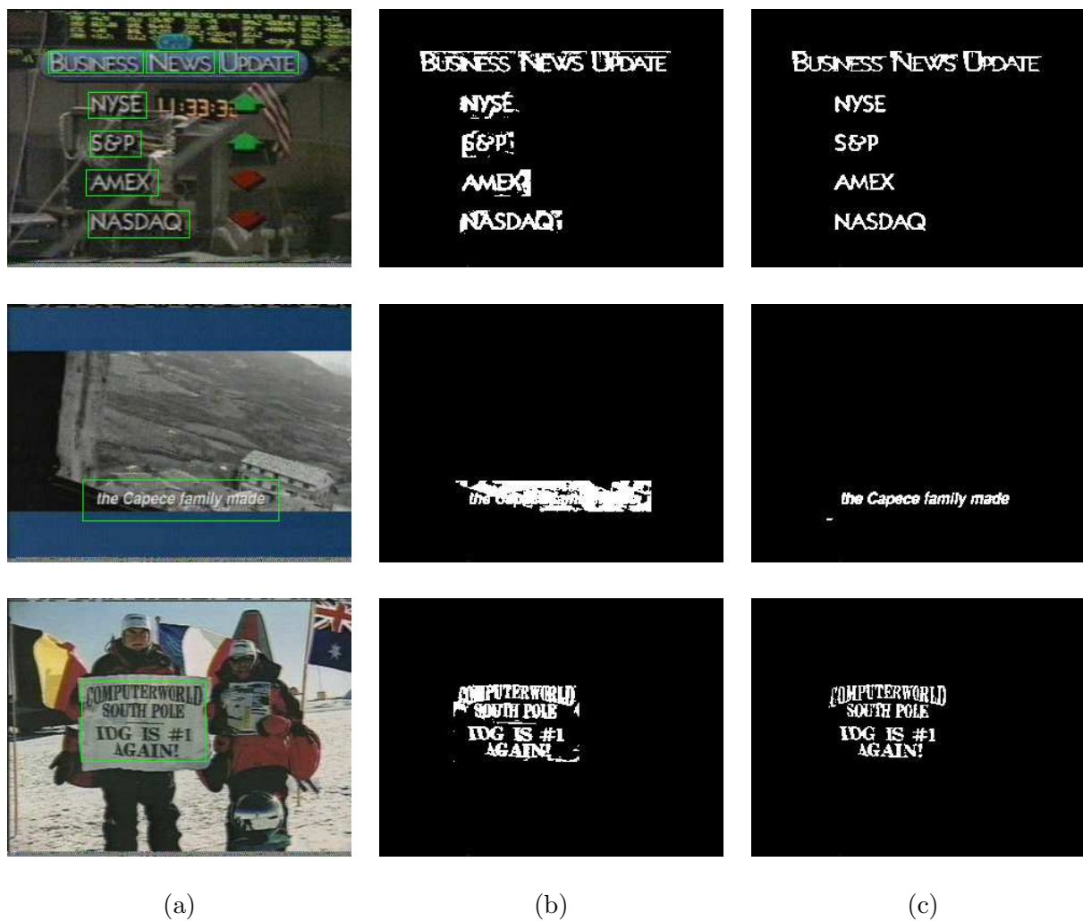
Fig. 4.5. Binarization results for sample video frames. (a): localized text regions; (b): output of binarization algorithm by Agnihotri et al [1]; (c): output of my binarization algorithm.
