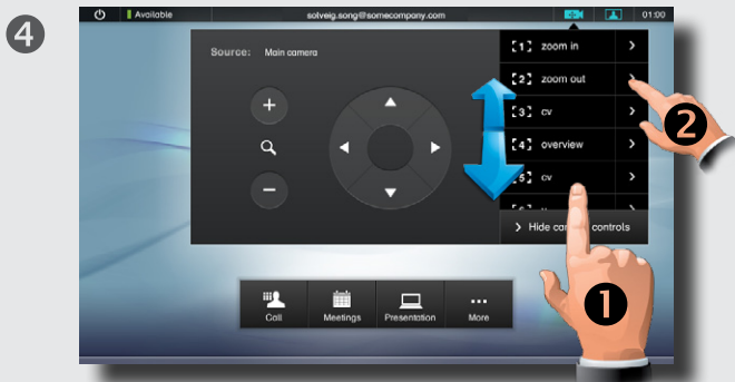
If needed, scroll to show the camera preset to be updated (1) and then tap > of that preset to expand the menu (2).
