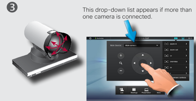
Using the expanded menu, adjust camera pan, tilt and zoom, as required. If you have more than one camera connected to your system, a drop-down list will let you choose which camera the preset will apply to.
