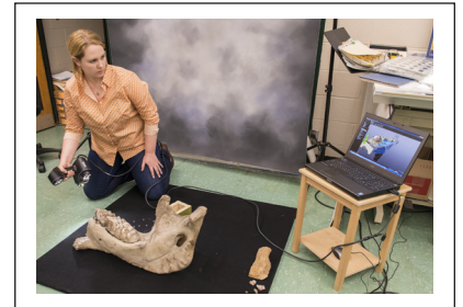
Figure 2: Here, a staff member is 3-D scanning the mastodon jawbone using a Creaform GoScan 50
