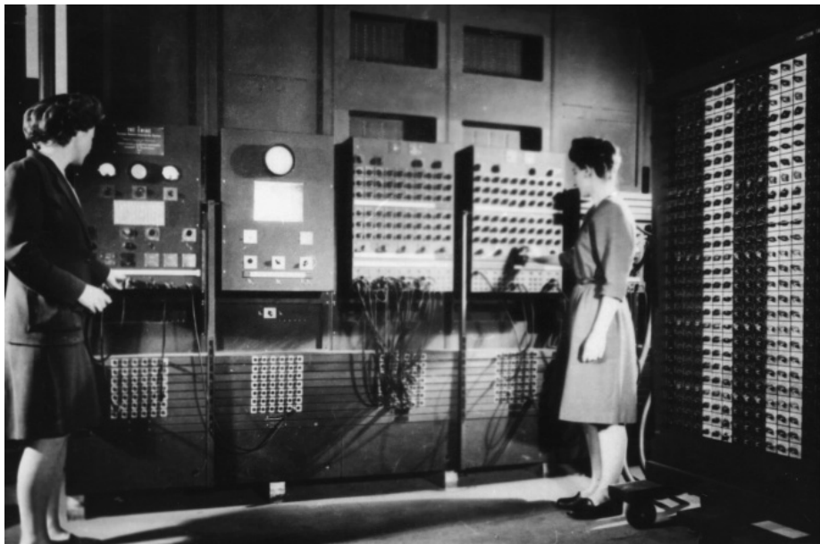
Figure 6.4. Programming ENIAC as telephone switching. Betty Jean Jennings Bartik (left) and Frances Bilas Spence (right) setting up the ENIAC at the Moore School. (U.S. Army Photo, http://ftp.arl.army.mil/~mike/comphist/ .)
