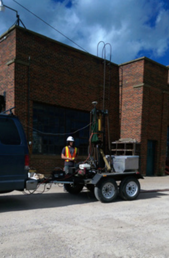
Images: Field photos showing weight drop source (top) and land streamer (bottom) in the vicinity of the Yates shaft at SURF.
