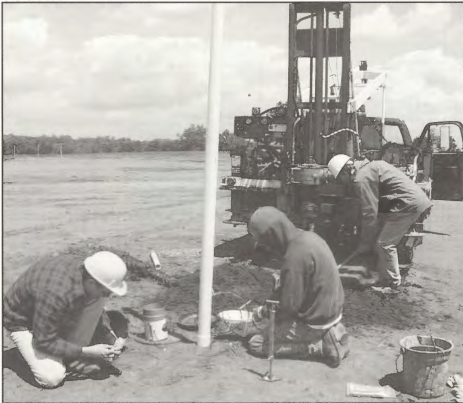
Pore water from a coal-processing waste pile at an abandoned Chinook coal mine in Clay County is collected for chemical analysis. Tracy Branam directs the project.
