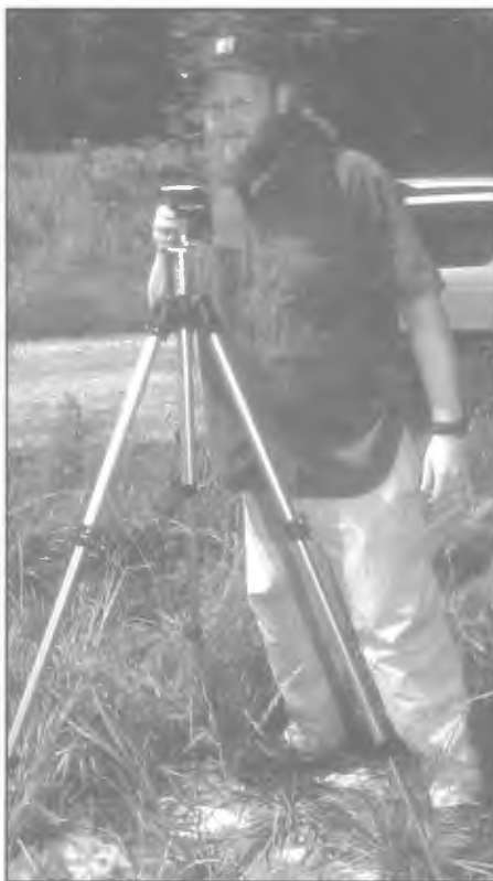
Chris Dintaman uses current map-grade technology (Trimble GeoExplorer II) to obtain coordinates of a landfill benchmark.
