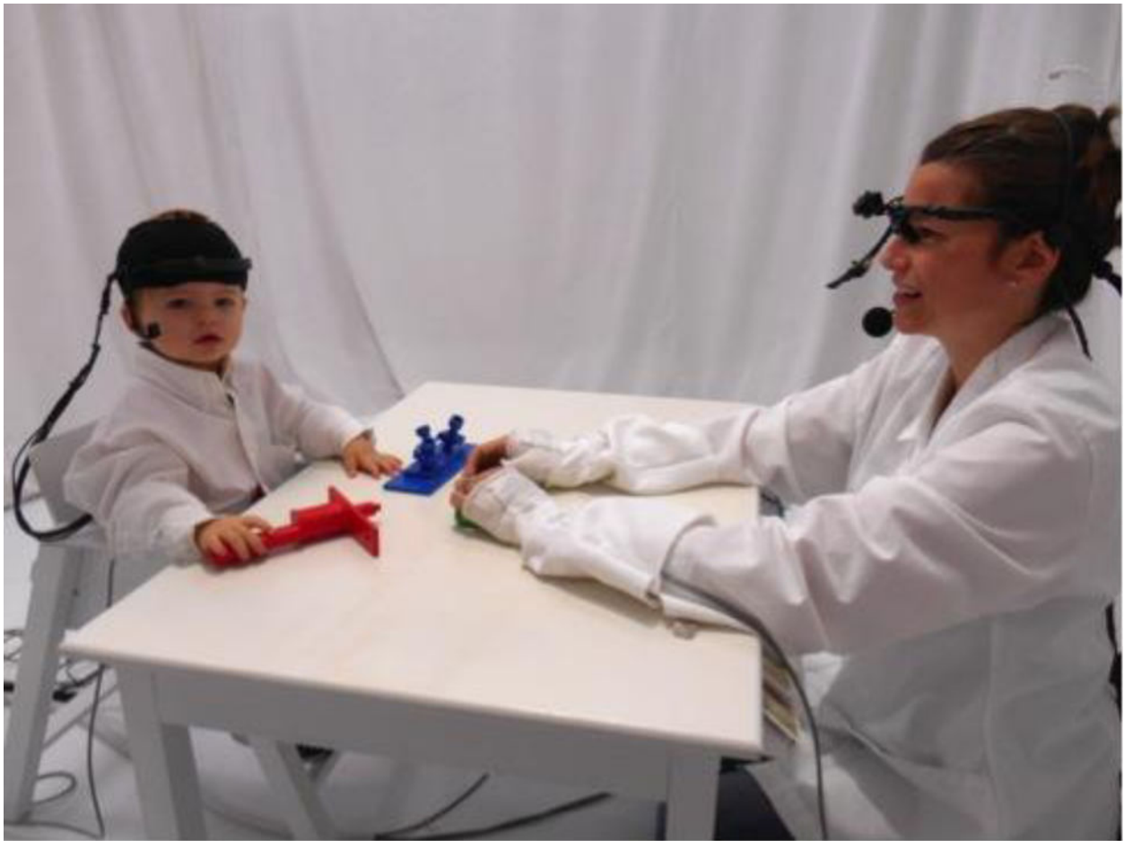
Figure 1. Parent and infant in the tabletop with novel objects and dual head-mounted eye-tracking. The authors received signed consent for the parent and infant's likenesses to be published in this article.
