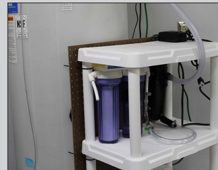
The 100-gallon ASW reservoir has a closed-circuit system for filtering and sterilizing the artificial seawater. Photo by Terri Greene
